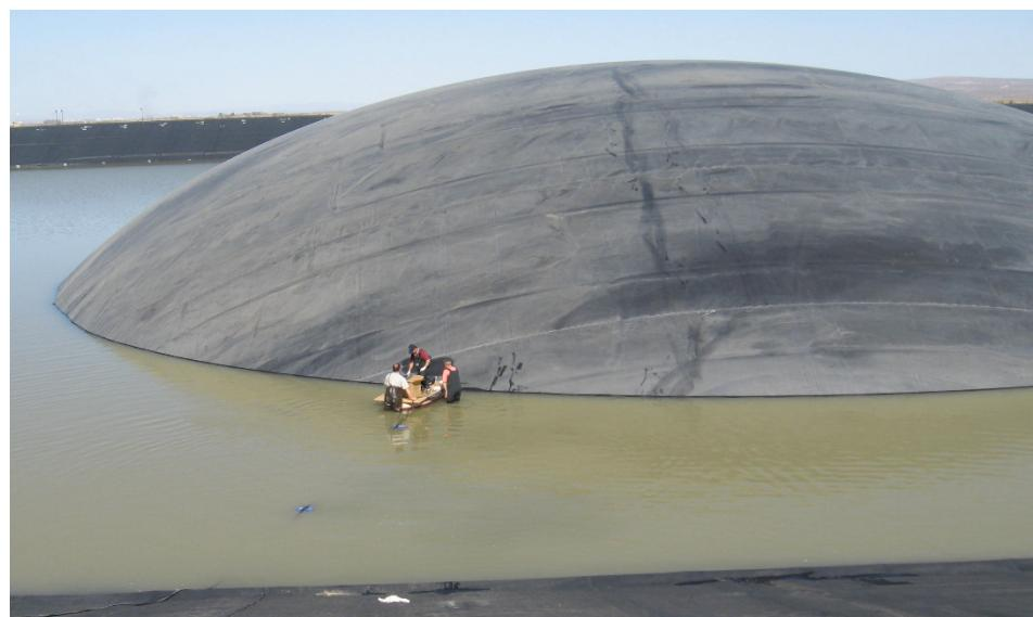
**Figure 3. Photo of real-world bubble indicative of calculations presented in the model. Note the people in the photo for scale.**
